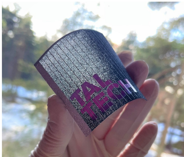
Fig. 1 Photo of the MGL solar cell prototype.
